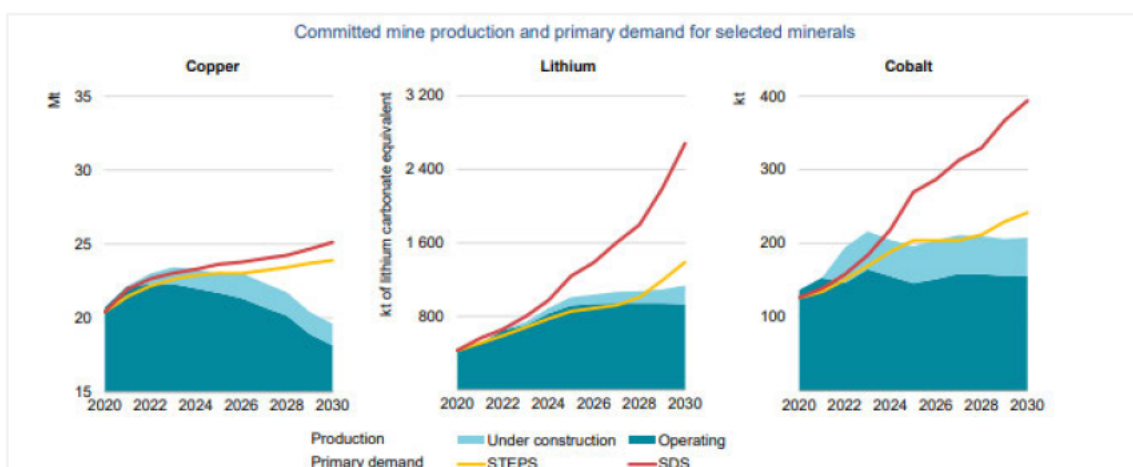
Figure 3. Production compared with demand for selected minerals under Stated Policies Scenario (STEPS) and Sustainable Development Scenario (SDS). IEA, Role of Critical Minerals in Clean Energy Transitions (2021)
