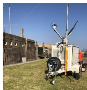
Figure 9: Trailer based solutions allow temporary broadcasts to rapidly deployed
