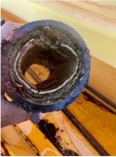
1. Sewer pipe showing build up
