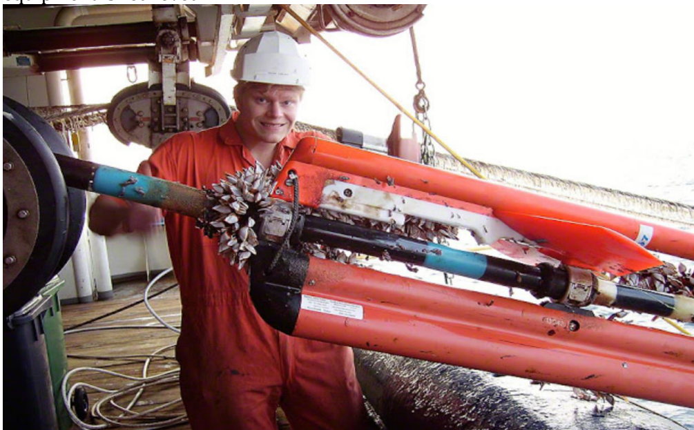
Fig 12. Barnacle growth on streamer depth controller.
