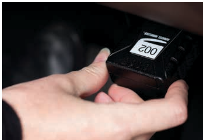
FIGURE 17. OBD-II GPS DEVICES WERE INSTALLED IN POST-2006 VEHICLE MODELS
