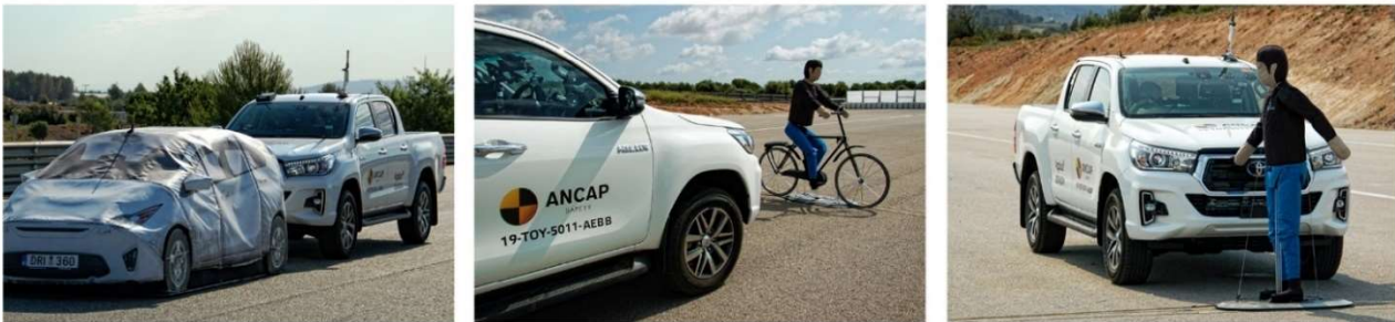
Figure 8 - AEB Scenarios: Car-to-Car rear, Car-to-Cyclist and Car-to-Pedestrian
