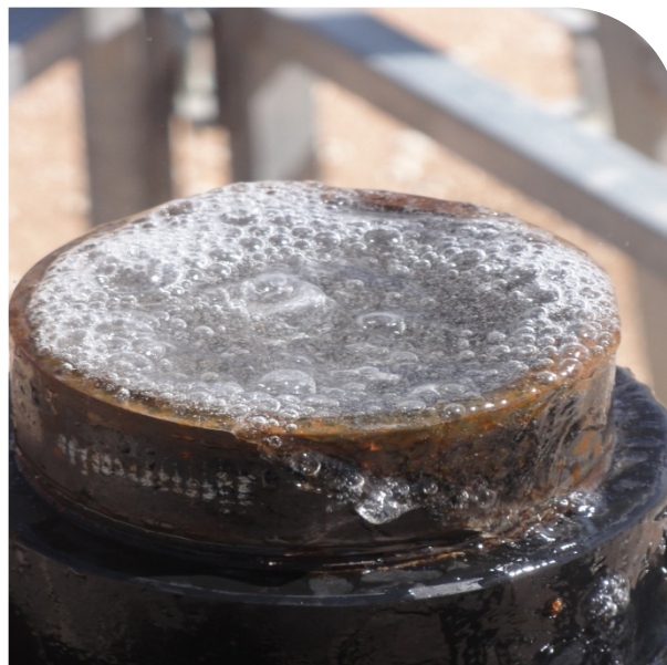
Naturally occurring methane can be seen producing bubbles in a groundwater monitoring bore. This bore is located in an area where CSG production is not yet taking place
