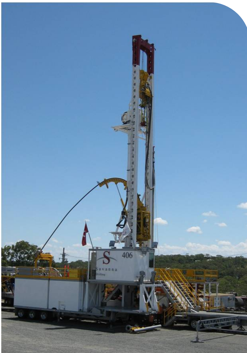
Australia Pacific LNG is using latest technology coiled tubing drilling rigs which will allow a significant reduction of drilling 'footprint' in agricultural areas
