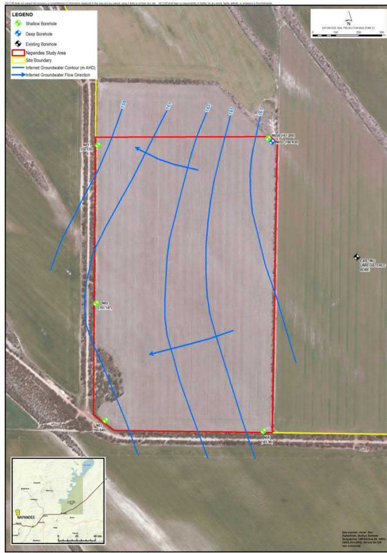
Figure 27 Interpreted Groundwater Contours and Inferred Flow Direction 23/05/18 – Watertable Aquifer Napandee
