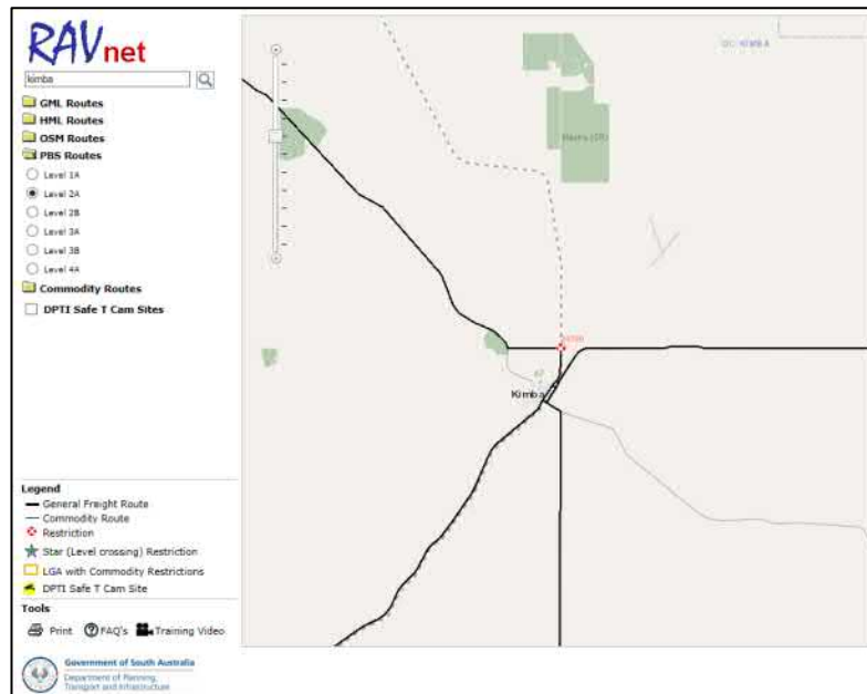
Figure 44 Approved restricted access vehicle routes approved under PBS Level 2A – 26m B-double (Department of Planning, Transport and Infrastructure, 2018)
