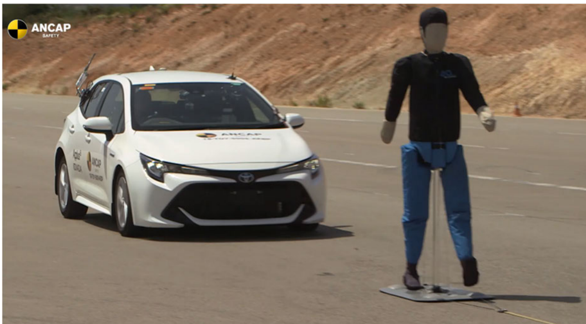
Figure 1 – The Toyota Corolla undergoing ANCAP AEB pedestrian testing
