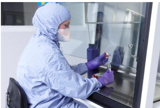
3. Compounding technicians wear special sterile garments to protect themselves from any spillage and to ensure the sterility of the product
