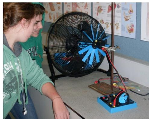
Figure 2. A STELR wind turbine in use.
