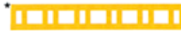
Holding position when Cat I, II or III precision approaches are being used.
