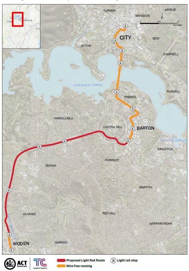
Figure 4.2 Overhead line power and wire-free running locations
