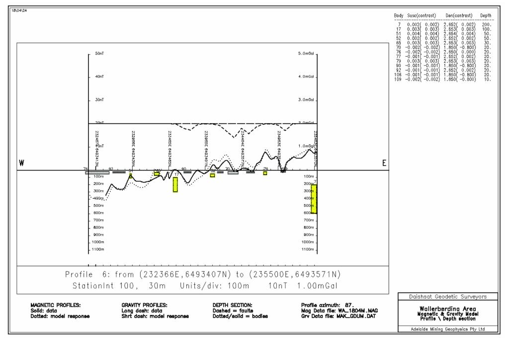
Figure A1. When Bodies 90, 70, 106 and 109 (magnetite depleted paleochannels?) are given a negative density contrast expected for unconsolidated cover the calculated gravity responses of the bodies (short dashed line) generate conspicuous troughs, which, if seen in gravity data would corroborate the paleochannel interpretation.
