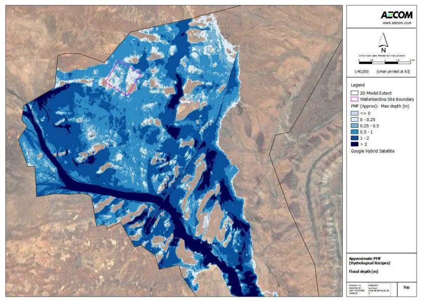
Figure 98 RFFE 1% AEP (5% lower confidence limit) flood depth
