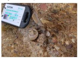
Comparison of sonic core sample from W04 (26.0 - 26.1 m bgs) with Hookina Waterhole outcrop – 10/05/18
