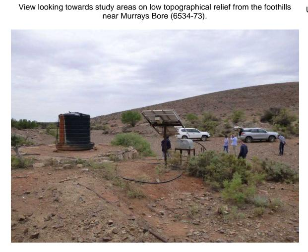
Close up of Murrays Bore set up. Water level was measured at 1.6 m below top of casing, total well depth was 39 m below top of casing on 21/02/18.
