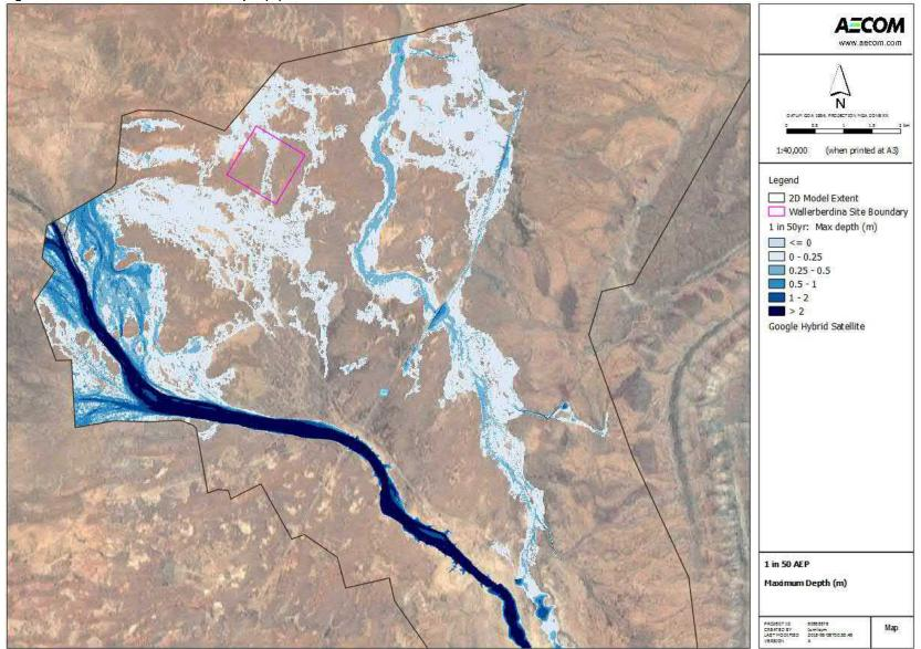
Figure 105 1 in 100 AEP Maximum Flood Depth (m)
