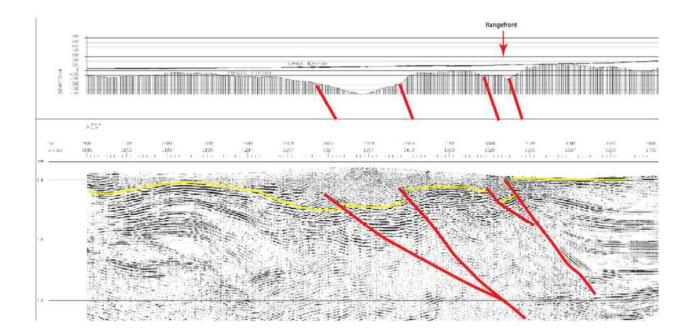
Seismic line 09TE-01 traverses the Ediacara scarp to the north of Wallerberdina (Figure 49). The interpretation of this line by Carr et al. (2010) confirms that the Ediacara fault is associated with a significant displacement of the Cenozoic section (66ma), whose base is shown by the yellow line. Similarly, the interpretation of seismic line 09GA-CG1 (Figure 50), located just south of Wallerberdina
