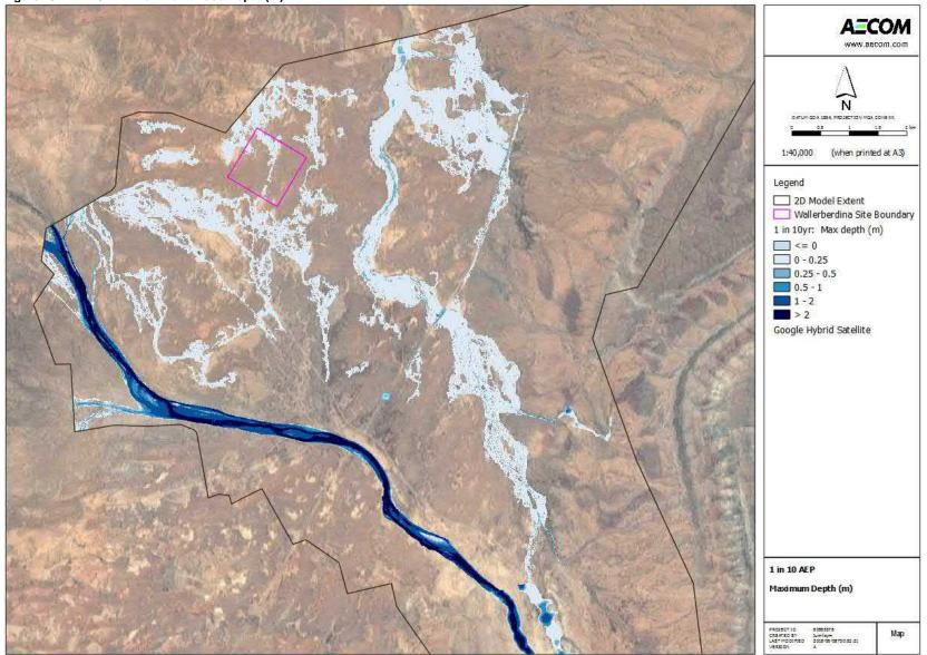
Figure 103 1 in 20 AEP Maximum Flood Depth (m)
