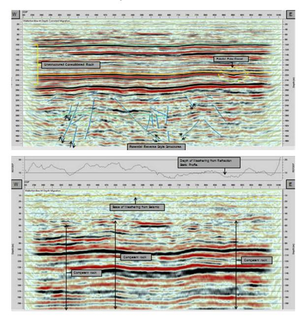
Figure 59 Wallerberdina North West 03 Depth Converted Migrated Stack Interpreted Structure (top) and Interpreted Section at Near Surface (bottom).
