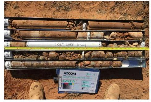
Figure 33 Core box showing intersected conglomerate at W02D
