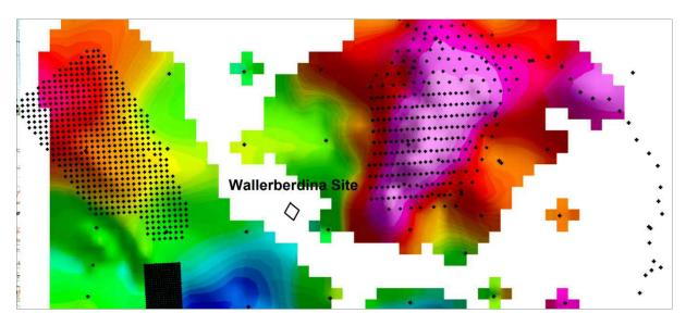
Image 3 Wallerberdina Bouguer Image showing gravity station coverage.
