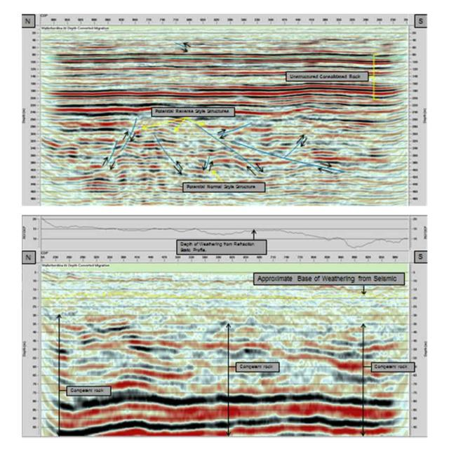
Figure 61 Wallerberdina South West 05 Depth Converted Migrated Stack Interpreted Structure (top) and Interpreted Section at Near Surface (bottom). Source: Velseis.
