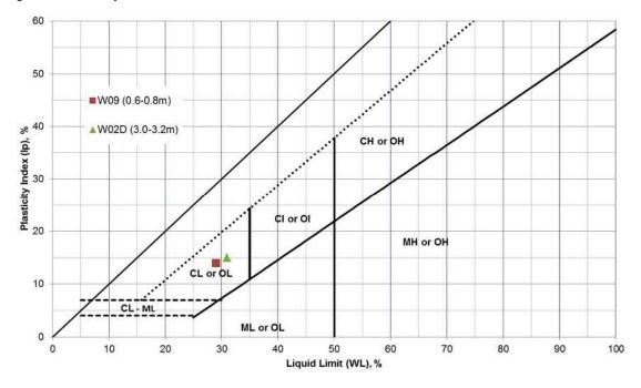
Figure 38 Plasticity Chart for Tested Materials
