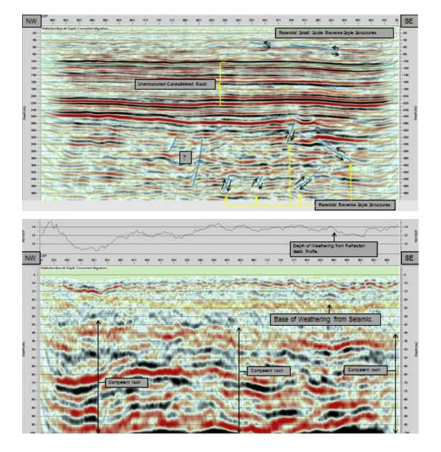
Figure 60 Wallerberdina South West 06 Depth Converted Migrated Stack Interpreted Structure (top) and Interpreted Section at Near Surface (bottom). Source: Velseis.
