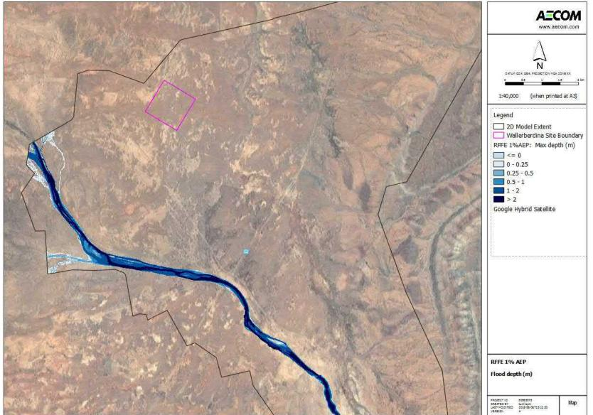
Figure 100 RFFE 1% AEP (95% upper confidence limit) flood depth
