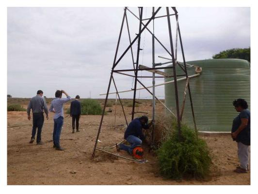
Well 6534-24, measured as dry at 24.8 m below top of casing on 21/02/18.
