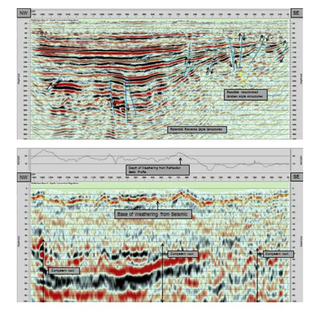
Figure 63 Wallerberdina East 01 Depth Converted Migrated Stack Interpreted Structure (top) and Interpreted Section at Near Surface (bottom). Source: Velseis.
