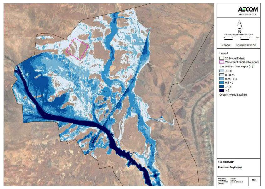
Figure 107 1 in 2000 AEP Maximum Flood Depth (m)
