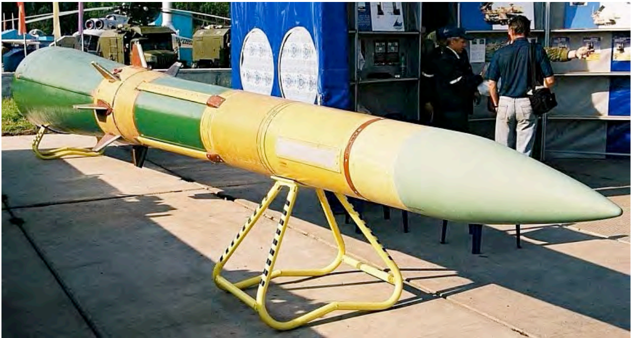
Hypersonic 9M82 / SA-12B GIANT missile, modelled on the Martin-Marietta Sprint missile. The Russian MoD has stated that the improved 9M82M variant has destroyed targets at 400 km range (M. Gyurosi).
