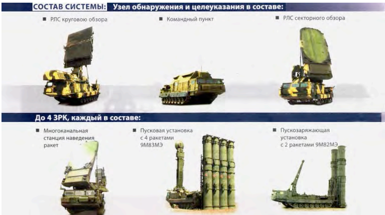
S-300VM/V4 / SA-23A/B Long Range SAM System battery components (Almaz-Antey).
