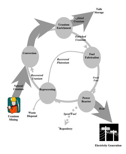
Accounting and tracking are necessary because uranium undergoes a number of processes, and produces new nuclear material, as it moves through the fuel cycle – see Figure 1:
