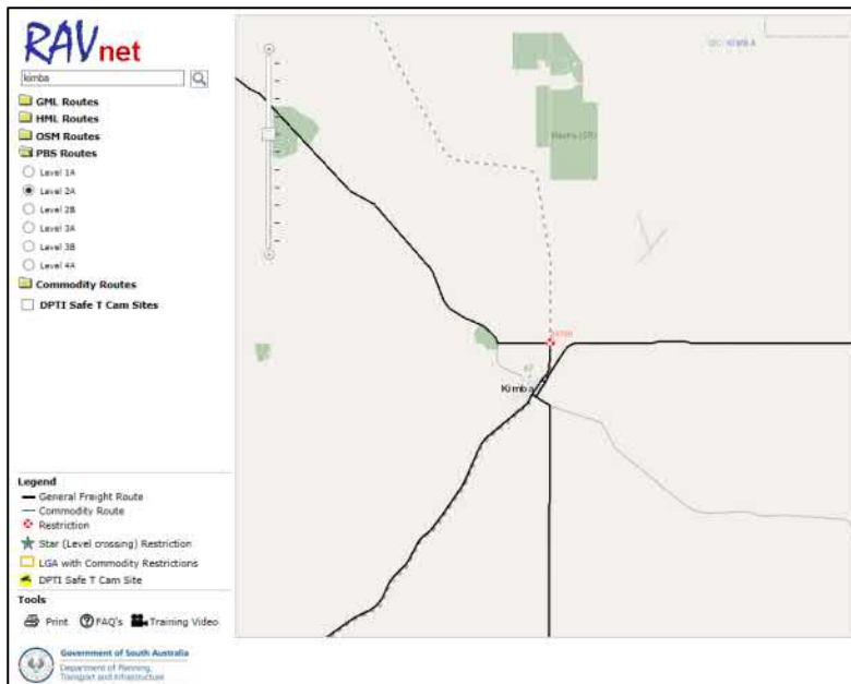
Figure 39 Approved restricted access vehicle routes approved under PBS Level 2A – 26m B-double (Department of Planning, Transport and Infrastructure, 2018)
