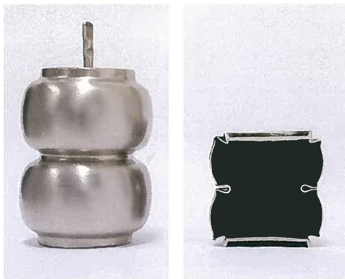
Synroc can and cut-away of the synroc wasteform.
